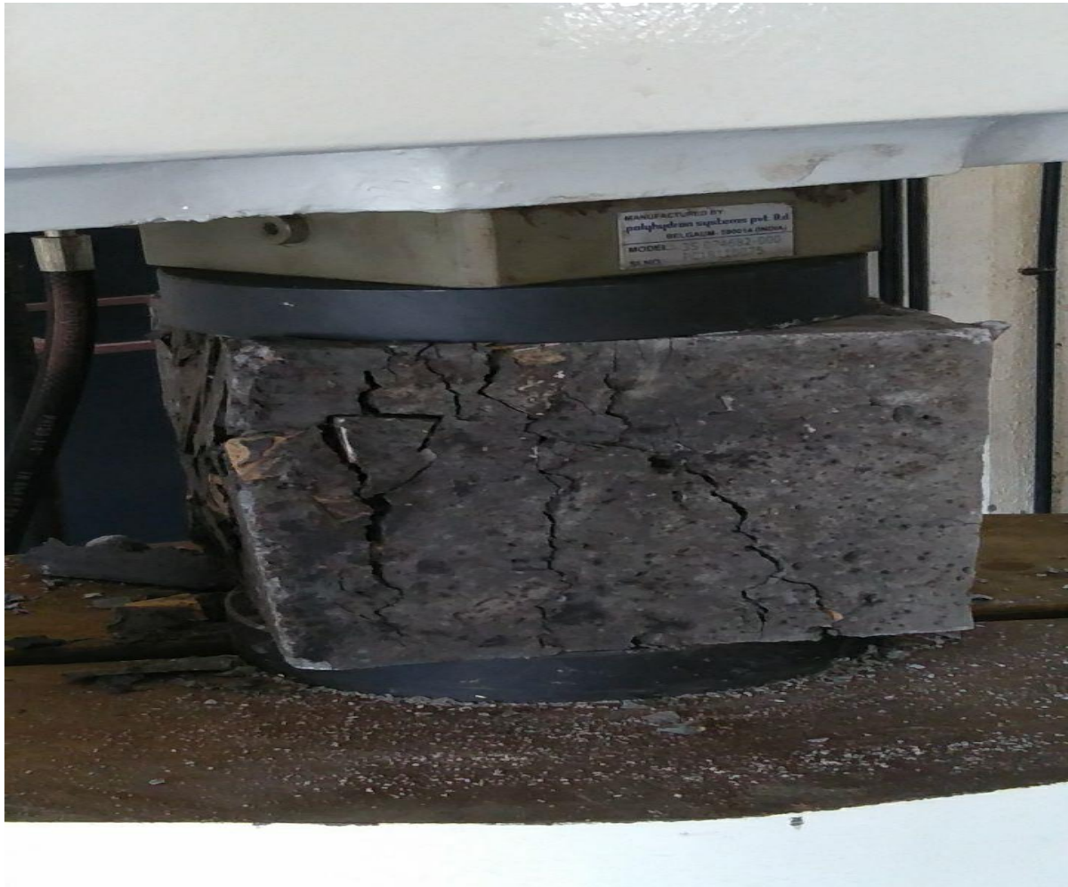
Fig 2: Compression test on UTM
