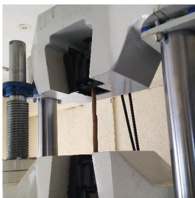
Fig -6: Bamboo Cylindrical Strip Tensile Test
