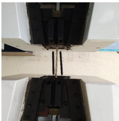
Fig -5: Bamboo Strip Tensile Test
