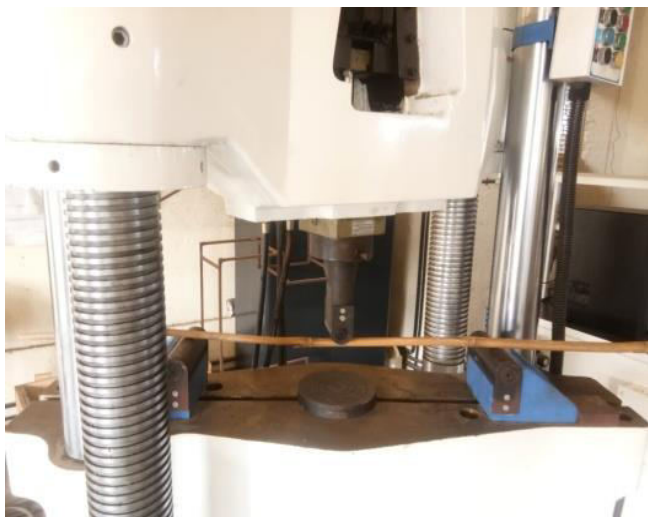
Fig -4: Hollow Cylindrical Bending Test
