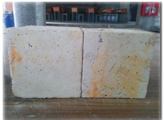
Fig 1: Hydrochloric Acid Attack on Concrete
