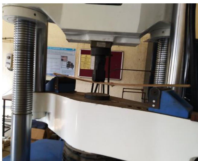
Fig -3: Bamboo Strip Bending Test
